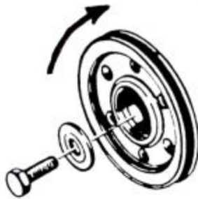
Lower Front Crank Pulley Can be rotated clockwise with a 19mm wrench on bolt, to align timing marks
